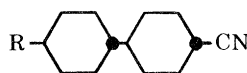
FIGURE 5. The general structure and an unusual pattern of behaviour for the bicyclohexyl compounds known as the CCH materials. Smectic properties diminish as R = alkyl increases in length.
